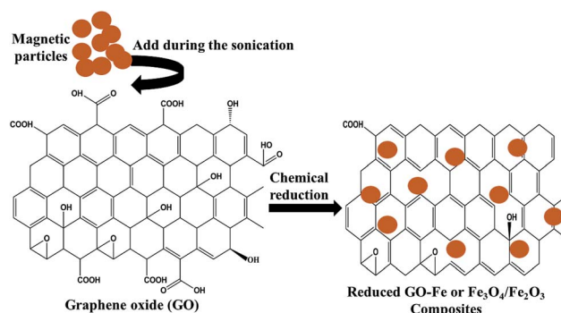
Fig. 12 Chemical reduction method of preparation for Fe and RGO based composites.
