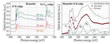
Fig. 6 (Left) Oxygen K-edge and iron L<sub>2,3</sub>-edge spectra of hematite samples of different thickness (accumulated over 1000 pulses). (Right) NEXAFS spectrum of hematite sample (thickness 35 nm) at the oxygen K-edge fitted with 6 Gaussian peaks (thin solid lines) and one arctan function (thin dashed line) in comparison to synchrotron data.<sup>33</sup> The samples have been provided by the group of F. de Groot (University of Utrecht, Netherlands)
