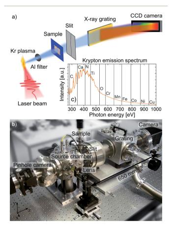
Fig. 1 (a) Schematic drawing and (b) photograph of the table-top setup for NEXAFS spectroscopy and (c) characteristic emission spectrum of the krypton plasma with accessible K- and L-shell absorption edges of prominent elements in the soft X-ray spectral range
