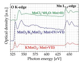
Fig. 5 Oxygen K-edge and manganese  $L_{2,3}$ -edge spectra of manganese dichloride (MnCl<sub>2</sub>·4H<sub>2</sub>O), manganese oxide/potassium manganate (MnO<sub>2</sub>/K<sub>2</sub>MnO<sub>4</sub>), and potassium permanganate (KMnO<sub>4</sub>) (accumulated over 10 000 pulses). For better visibility the spectra are shifted along the *y*-axis.
