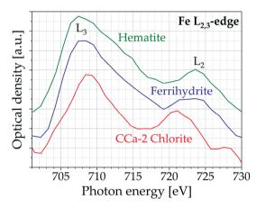
Fig. 7 Iron  $L_{2,3}$ -edge spectra of hematite, ferrihydrite and CCa-2 chlorite (accumulated over 1000 pulses). For better visibility the spectra are shifted along the y-axis
