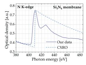
Nitrogen K-edge spectrum of a Si<sub>3</sub>N<sub>4</sub> membrane (thickness 100 nm, accumulated over 1000 pulses) in comparison to tabulated data.27
