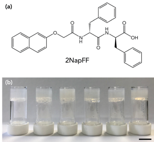
Fig. 1 (a) Chemical structure of gelator 2NapFF. (b) Photographs of 2NapFF at (left to right) 10 mg mL -1 , 5 mg mL -1 , 2.5 mg mL -1 , 20 : 80 glycerol : water (5 mg mL -1 ), 40 : 60 glycerol : water (5 mg mL -1 ) and 60 : 40 glycerol : water (5 mg mL -1 ). Scale bar is 1 cm.
