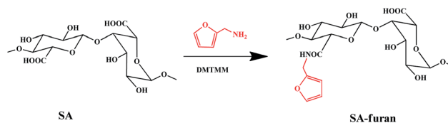
Scheme 1 Synthesis steps of SA-furan.
