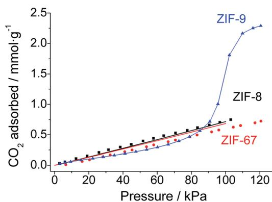
Fig. 2 Experimental CO<sub>2</sub> adsorption isotherms at 25 °C of the powdered cobalt-based materials ZIF-9 (blue triangles) and ZIF-67 (red circles), compared with the ZIF-8 CO<sub>2</sub> isotherm (black squares) reported by Zornoza *et al.*<sup>56</sup> Solid lines show simulated ZIF-8 (black) and ZIF-67 (red) isotherms with a good fit to the experimental data (filled symbols). The solid line in the ZIF-9 isotherm is a guide to the eye.
