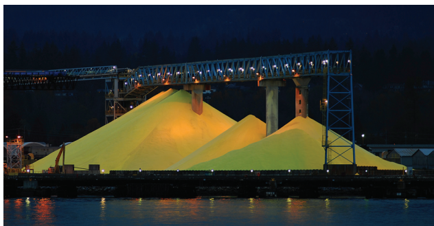
Fig. 2 A stockpile of sulfur produced from the hydrodesulfurisation process in petroleum refining. Approximately 70 million tonnes of sulfur were produced in 2015 by the petroleum industry. Image credit: Gord McKenna, made available through a Creative Commons license: https://www.flickr.com/photos/gord99/5170487123/ .
