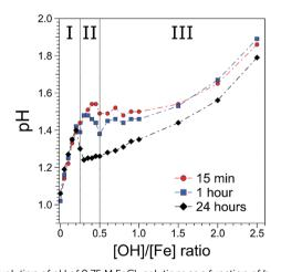
Fig. 1 Evolution of pH of 0.75 M FeCl $_3$  solutions as a function of h = [OH]/[Fe] ratio. Regions I–III correspond to the transitions from monomeric iron species to iron-oxo oligomers, and finally iron-oxo solid particles. Region I: oligomers with <1 nm diameter. Region II: cylindrical particles. Region III: cylindrical particles and akaganeite formation.
