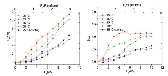
Fig. 3 (a) Friction force and (b) effective friction coefficient,  $\mu_{\rm eff} = F_{\rm f}/F_{\rm n}$ , as a function of applied normal load between silica surfaces carrying a preadsorbed layer of PIPOZ<sub>60</sub>-b-PAMPTMA<sub>17</sub> measured at different temperatures. Reproduced with permission from ref. 16. Copyright, 2017 American Chemical Society.
