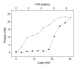
Fig. 4 An example of a friction vs. load cycle measured between DPPC bilayers on silica surfaces across 150 mM PBS buffer solution. In this case the bilayer was compromised at a load of just below 20 nN. Friction forces measured on loading and unloading are shown with filled ( ) and unfilled (O) symbols, respectively. The temperature was 25 °C. Reprinted with permission from ref. 37. © 2017 Elsevier Inc.
