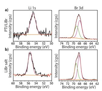
Fig. 10 Li1s and Br3d XPS spectra of crystalline (a) PTI-LiBr and (b) LiBr.
