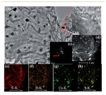
Fig. 2 TEM images (a), HRTEM image (b), SAED pattern (c), HAADF-STEM (d) and elemental mapping images (e-h) of  $Co_3S_4-S/G-800$ catalyst.
