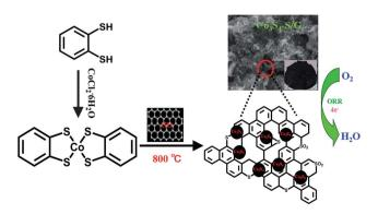
Fig. 1 Schematic illustration of the fabrication process of  $\text{Co}_3\text{S}_4-\text{S}/\text{G}$  catalysts and electrocatalytic activity for oxygen reduction reaction.
