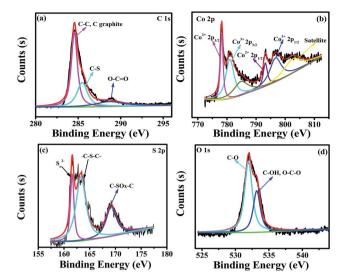
Fig. 3 High-resolution C 1s XPS spectra (a), Co 2p spectra (b), S 2p spectra (c) and O 1s spectra (d) of the as-obtained Co<sub>3</sub>S<sub>4</sub>-S/G-800 hybrids.
