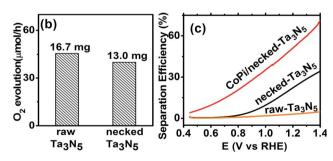
Fig. 4 (a) Schematic comparison of  $O_2$  evolution processes via photocatalysis (AgNO $_3$  as electron scavenger) and photoelectrocatalysis. (b) Photocatalytic activity of the  $Ta_3N_5$  powder peeled from raw- $Ta_3N_5$  and necked- $Ta_3N_5$  electrodes. The mass of the photocatalyst is listed above the column, respectively. (c) Charge separation efficiency of raw- $Ta_3N_5$  (orange), necked- $Ta_3N_5$  (black) and CoPi/necked- $Ta_3N_5$  electrodes (red).
