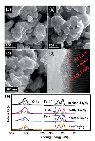
Fig. 1 SEM images of (a) raw- $Ta_3N_5$  electrode, (b)  $TaCl_5-Ta_3N_5$ electrode, and (c) necked-Ta<sub>3</sub>N<sub>5</sub> electrode. (d) HRTEM image of necked-Ta<sub>3</sub>N<sub>5</sub> electrode. (e) XPS spectra of O 1s and Ta 4f for raw-Ta<sub>3</sub>N<sub>5</sub> (orange), heated-Ta<sub>3</sub>N<sub>5</sub> (blue), TaCl<sub>5</sub>-Ta<sub>3</sub>N<sub>5</sub> (pink) and necked-Ta<sub>3</sub>N<sub>5</sub> (black) electrodes.
