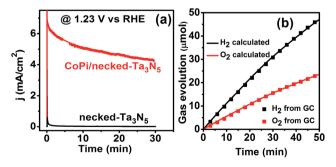
Fig. 7 (a) Stability of the necked- $Ta_3N_5$  (black) and CoPi/necked- $Ta_3N_5$  (red) photoanodes at 1.23 V vs. RHE. (b) Faradaic efficiency of the CoPi/necked- $Ta_3N_5$  photoanode at 1.23 V vs. RHE. Electrolyte: 1 M NaOH aqueous solution. Illumination: 100 mW cm<sup>-2</sup>, Xe lamp (wavelength > 420 nm), area: 0.6 cm<sup>2</sup>.
