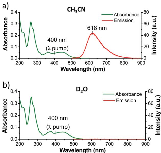
Fig. 3 UV/Vis absorption and emission spectra ( $\lambda_{\text{ex}} = 410 \text{ nm}$ ) of **1** ( $3.0 \mu\text{M}$ ) in (a)  $\text{CH}_3\text{CN}$  and (b)  $\text{H}_2\text{O}$ , showing the solvent dependent luminescence of **1**. The excitation wavelength for the TRIR experiments is also highlighted.
