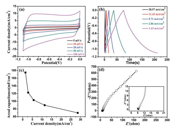
Fig. 4 (a) CV curves at different scan rates; (b) GCD curves at different current densities of the helical MoO<sub>2</sub> in 1.0 M Na<sub>2</sub>SO<sub>4</sub> electrolyte; (c) areal capacitance calculated from GCD curves as a function of current densities; (d) EIS spectra of MoO<sub>2</sub> (inset is the enlarged view of the high frequency region).
