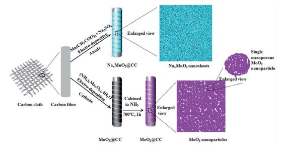
Scheme 1 Representation of the fabrication of the helical hierarchical porous Na<sub>x</sub>MnO<sub>2</sub>/CC and MoO<sub>2</sub>/CC
