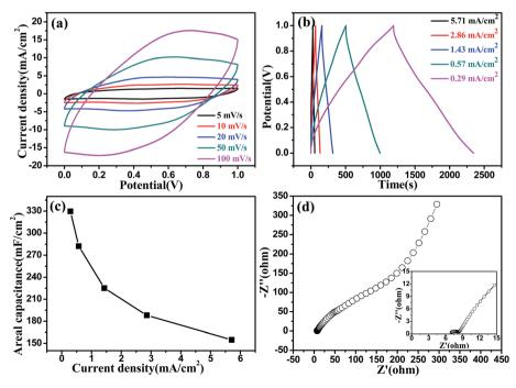
Fig. 2 (a) CV curves of the helical  $Na_xMnO_2$  at different scan rates; (b) GCD curves of the helical  $Na_xMnO_2$  at different current densities in 1.0 M Na<sub>2</sub>SO<sub>4</sub> electrolyte; (c) areal capacitance calculated from GCD curves as a function of current densities; (d) EIS spectra of the Na<sub>x</sub>MnO<sub>2</sub> (inset is the enlarged view of the high frequency region).
