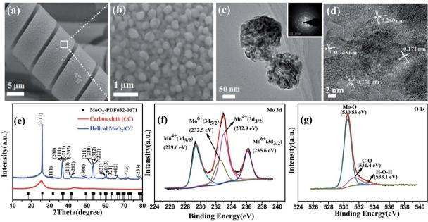
Fig. 3 (a and b) SEM images of the helical  $MoO_2$  with different magnifications; (c) the TEM image of  $MoO_2$  nanoparticles (inset is the SAED pattern); (d) the HRTEM image of the helical  $MoO_2$ ; (e) XRD patterns of the helical  $MoO_2$ /CC and CC; XPS spectra of the helical  $MoO_2$ /CC: (f) Mo 3d and (g) O 1s.
