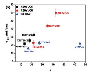
Fig. 4 Hydroxide conductivity of membranes as a function of (a) IEC (ion exchange capacity) and (b) hydration number  $\lambda$  (moles of water per mole of quaternary ammonium group) in water at room temperature. Conductivities were measured with samples exposed to liquid water.
