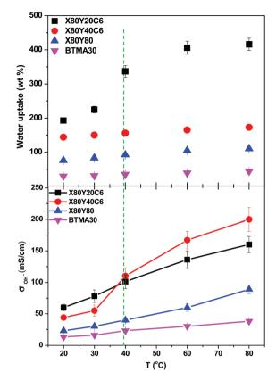
**Fig. 5** Hydroxide conductivity of X80YxC6 and BTMA30 membranes as a function of temperature. Conductivities were measured with samples exposed to liquid water.
