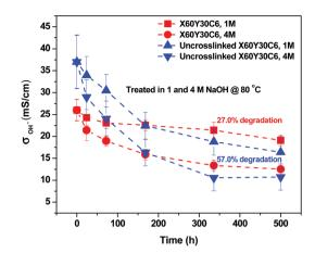
Fig. 8 Chemical stability of the quaternary ammonium cation of X60Y30C6 and uncross-linked X60Y30C6 in 1 M and 4 M NaOH solutions, respectively, at 80 °C, and OH conductivity as a function of duration time measured at 20 °C.
