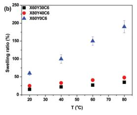
Fig. 3 Liquid water uptake (a) and swelling ratio (b) of membranes in the OH<sup>-</sup> form as a function of temperature
