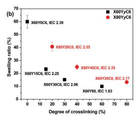
Fig. 2 Liquid water uptake (a) and swelling ratio (b) of membranes in the OH<sup>-</sup> form as a function of degree of cross-linking at room temperature.
