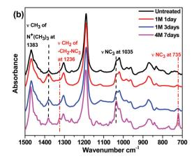
Fig. 9 ATR spectra of the treated X60Y15C6 membrane. (a) ATR spectra of the functional group region and (b) fingerprint region.
