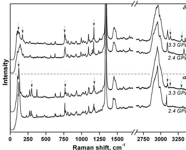
Fig. 4 Raman spectra of the  $\alpha$ - and  $\delta$ -polymorphs of chlorpropamide providing evidence of the phase transitions in the pressure change from 2.4 to 3.3 GPa. The most significant changes in the Raman spectra are shown by arrows and are mainly related to lattice vibrations ( $50\text{--}350\text{ cm}^{-1}$ ), CC and SO stretching vibrations ( $750\text{--}1250\text{ cm}^{-1}$ ) and rearrangements of H-bonds ( $3050\text{--}3360\text{ cm}^{-1}$ ).
