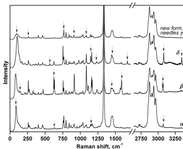
**Fig. 3** Raman spectra of the  $\alpha$ -,  $\beta$ -, and  $\delta$ -polymorphs of chlorpropamide and the new needle-shaped ( $\gamma$ ) polymorph at the first pressure point (0.3 GPa). No solid-state transformations occur in the starting  $\alpha$ - and  $\delta$ -forms at this pressure. Characteristic features of the spectra for the different polymorphs are shown by arrows.
