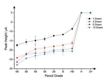
Fig. 3 Plots of pencil composition/grade vs. peak height (cathodic current) recorded in 1 mM hexaammineruthenium(III) chloride/0.1 M KCl as a result of increasing the number of draws. Scan rate: 50 mV s<sup>-1</sup> (vs. SCE). Data shown is an average and corresponding standard deviation (N = 3).
