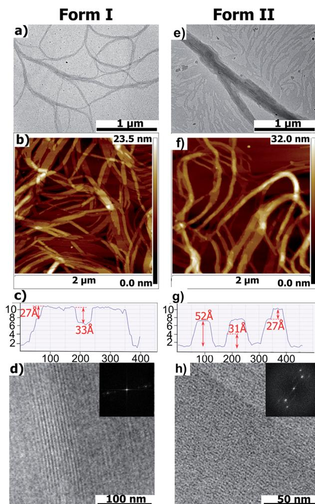
Fig. 2 Morphology of PBI-C10 in Form I and II. (a) & (e) TEM bright field images; (b) & (f) AFM images; (c) & (g) section profile of an AFM topographic image showing the presence of characteristic terraces; (d), (h) low dose HR-TEM images (inset: fast Fourier transform). In Form II, note the presence of some intense reflections in the first layer line above the equator which is a fingerprint of a helical molecular packing.
