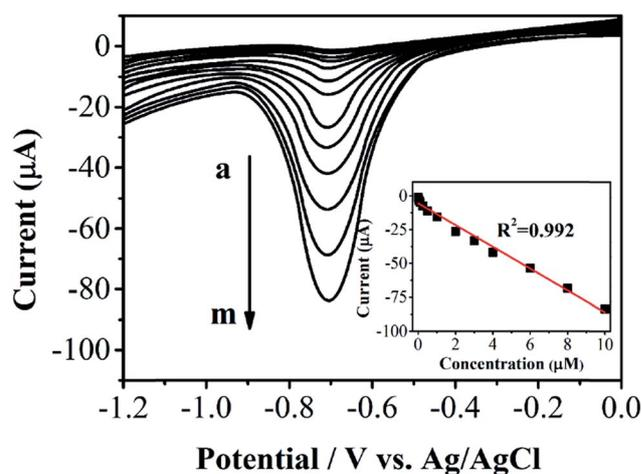
Fig. 5 DPV curves for phoxim at RGO–Au/GCE with different concentrations of phoxim (from a to m:  $0.008$ ,  $0.02$ ,  $0.05$ ,  $0.1$ ,  $0.25$ ,  $0.5$ ,  $1$ ,  $2$ ,  $3$ ,  $4$ ,  $6$ ,  $8$ ,  $10 \mu\text{M}$ ).
