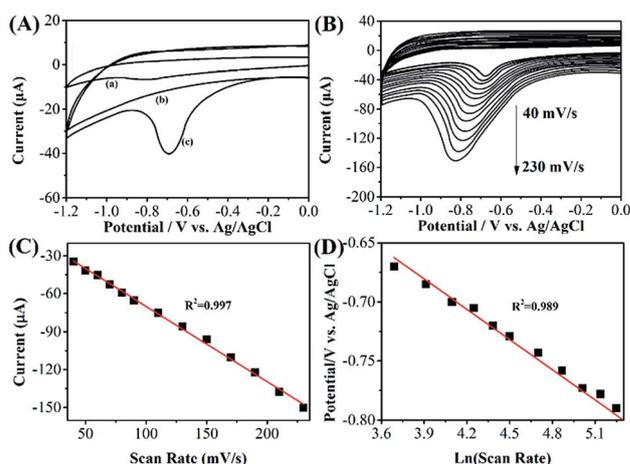
Fig. 3 (A) CVs of bare (a) GCE, (b and c) RGO-Au/GCE in  $0.1\text{ M}$  PBS (pH 7.0) with and without  $10\text{ }\mu\text{M}$  phoxim. Scan rate:  $50\text{ mV s}^{-1}$ . (B) CVs of RGO-Au/GCE in  $10\text{ }\mu\text{M}$  phoxim at different scan rates ( $40, 50, 60, 70, 80, 90, 110, 130, 150, 170, 190, 210$  and  $230\text{ mV s}^{-1}$ ). (C) The plot for the dependence of peak current on the scan rate. (D) The relationship between  $E_{pa}$  and  $\ln \nu$ .
