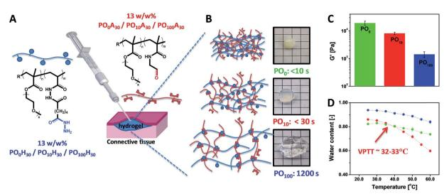
Fig. 6 (A) Preparation of POEGMA hydrogels using a double-barrel syringe. (B) Physical appearance and gelation time for  $PO_0$ ,  $PO_{10}$  and  $PO_{100}$  hydrogels. (C) Hydrogel mechanics as measured by the shear storage modulus (G'). (D) Thermoresponsive properties of  $PO_0$ ,  $PO_{10}$  and  $PO_{100}$  hydrogels. Data reproduced from ref. 42 with permission from Elsevier.
