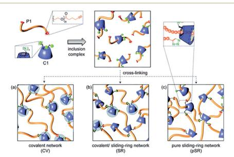
Fig. 1 Schematic representation of the formation of  $\alpha$ -cyclodextrin ( $\alpha$ CD)-polyethylene glycol(PEG) hydrogels through the formation of alkyneazide chemistry (CV), inclusion complexes (pSR) and a combination of both (SR). Reproduced from ref. 95 with permission from RSC Publishing.
