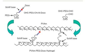
Fig. 4 Schematic representation of the formation of poly(vinylamine) (PVAm)–poly(ethylene glycol) (PEG)–doxorubicin(doxo) hydrogels using Schiff base chemistry. Reproduced from ref. 52 with permission from SAGE journals.
