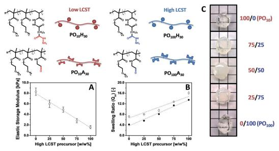
Fig. 7 Tuning hydrogel properties by mixing POEGMA precursors of different LCST. (A) Elastic storage modulus (G'), (B) mass-based swelling ratio ( $Q_m$ ) and (C) physical appearance of POEGMA hydrogels containing 100/0, 75/25, 50/50, 25/75 and 0/100 w/w% PO<sub>10</sub>H<sub>30</sub>/PO<sub>100</sub>H<sub>30</sub> and PO<sub>10</sub>A<sub>30</sub>/PO<sub>100</sub>A<sub>30</sub>. Data reproduced from ref. 155 and 157 with permission from Wiley-VCH and ACS.
