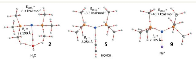
Fig. 4 Computer aided renderings of 2, 5, and 9, computed at the BP86-D3/def2-TZVP level of theory. The small red dots denote the bond-critical points according to an AIM analysis.
