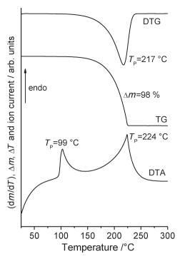
Fig. 11 DTA, TG and DTG curve for form 1t at 4  $^{\circ}\text{C}$  min  $^{-1}$  in a nitrogen atmosphere.
