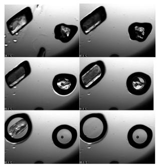
Fig. 13 Microscopic images at various temperatures (36.1, 87.5, 90.5, 91.5. 92.5. 93.5 °C) obtained by thermomicroscopy with form 1t (crystal on left) and form 10 (crystal on right).
