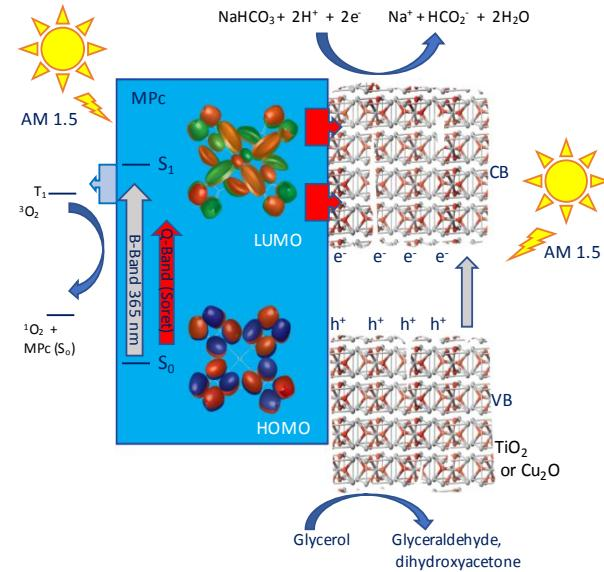
**Figure 1.** Schematic of the electron-transfer and redox chemical pathways via solar irradiation using semiconductor and MPC on quartz disc.
