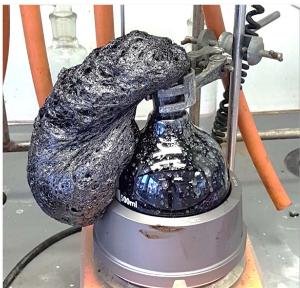
Fig. 4 Photograph of an inverse vulcanisation reaction after the effects of auto-acceleration. The reaction was carried out by heating 50 g of dicyclopentadiene and 50 g of sulfur at 140 °C in a 500 ml flask. Before the point where auto-acceleration occurred, the reaction mixture consisted of ~100 ml of smooth liquid being stirred and heated. After the heat generated by the exothermic reaction became too great to be lost to the surroundings, the mixture bubbled up rapidly – changing from a calm liquid to the form seen in approximately 2 seconds.
