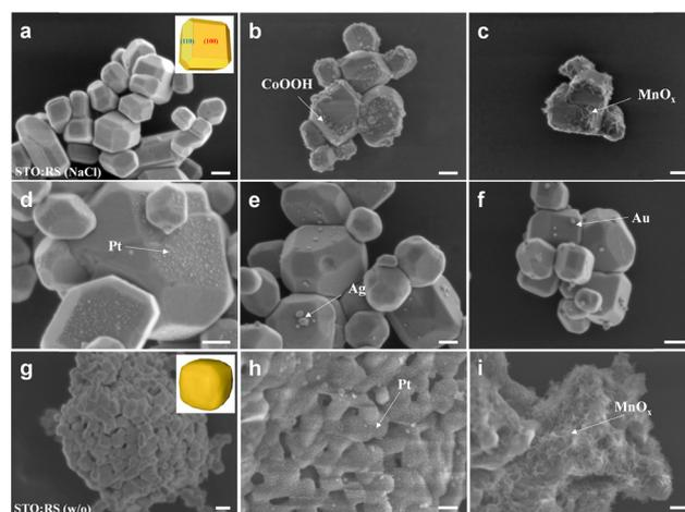
Fig. 2 SEM images of (a) STO:RS(NaCl) and STO:RS(NaCl) loaded with (b) CoOOH, (c) MnO<sub>x</sub>, (d) Pt, (e) Ag, and (f) Au by photodeposition. SEM images of (g) STO:RS(w/o) and STO:RS(w/o) loaded with (h) Pt and (i) MnO<sub>x</sub> by photodeposition; the scale is 100 nm.
