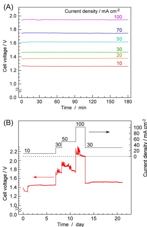
Fig. 4 Time courses of cell voltage for NH<sub>3</sub> synthesis from H<sub>2</sub>O and N<sub>2</sub> at various current densities and 250 °C. A summary of short-term current fluctuations (A) and the results obtained over a period of three weeks of operation (B). Note that (A) and (B) represent the experimental results from different cells that were reassembled, so the results do not perfectly match.
