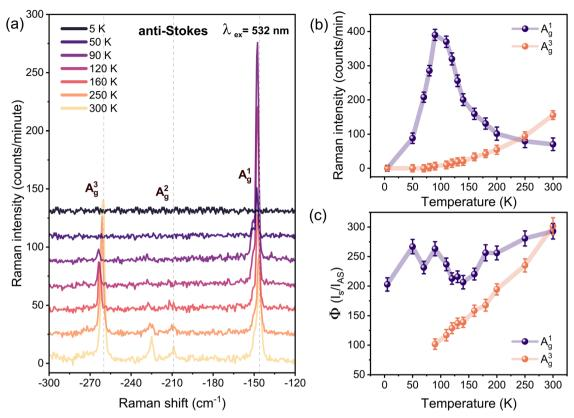
Fig. 4 (a) Temperature-dependent Raman anti-Stokes spectra of bulk PdSe<sub>2</sub> under parallel configuration (xx) with an excitation energy of 2.33 eV (532 nm). (b) Anti-Stokes Raman spectral weight intensities, as a function of temperature, of the  $A_{q'}^1$  and  $A_{q'}^3$  modes. (c) The calculated phonon temperature  $\phi(l_S/l_{AS})$  under non-resonance conditions for  $A_q^1$  and  $A_q^3$  phonon modes plotted as a function of temperature.
