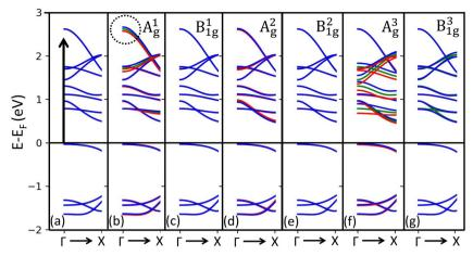
Fig. 7 Estimating the electron-phonon coupling using DFT calculations for the electronic dispersion of bulk PdSe<sub>2</sub> considering (a) unperturbed (green lines) and (b-g) different frozen phonons (blue and red for opposite displacements) (b)  $A_{q_1}^1$ , (c)  $B_{1q_1}^2$ , (d)  $A_{q_1}^2$ , (e)  $B_{1q_2}^2$ , (f)  $A_{q_1}^3$ , and (g)  $B_{1q_2}^3$ .
