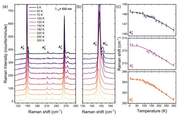
Fig. 2 (a) and (b) Temperature-dependent Raman spectra of bulk PdSe<sub>2</sub> under parallel configuration (xx), with an excitation energy of 2.33 eV (532 nm). (c) Raman frequencies as a function of temperature for the  $A_q^1$ ,  $A_q^2$ , and  $A_q^3$  phonon modes. In each panel, we fit the data to the anharmonic model characterized by the processes of optical phonon decay (solid lines) using eqn (1) over the entire temperature range 5 to 300 K.
