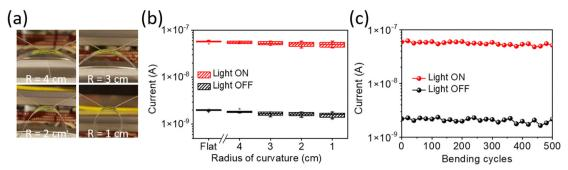
Fig. 6 (a) Photograph of the flexible MQDs@10/CNF paper photodetector under different bending conditions. (b)  $I_{on}$  and  $I_{off}$  of the MQDs@10/CNF photodetector measured with various bending curvature from flat, 4, 3, 2, to 1 cm. (c) Endurance characterization of the MQDs@10/CNF device.
