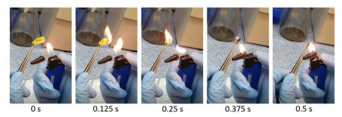
Fig. 7 Time-lapse sequence of photographs showing the ignition process of the MQDs/CNF paper photodetector within 0.5 s.
