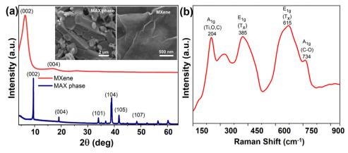
Fig. 1 (a) XRD spectra of MAX phase and MXene, inset figures show SEM images that depict their morphology. (b) Raman spectrum of MXene
