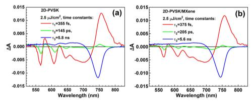
Fig. 7 Wavelength-dependant amplitudes of the indicated time constants from a 3-exponential global fit of TA data excited from HTL side at 475 nm with 2.5  $\mu$ J cm<sup>-2</sup> pump fluence for the cells: (a) without MXene and (b) with MXene.
