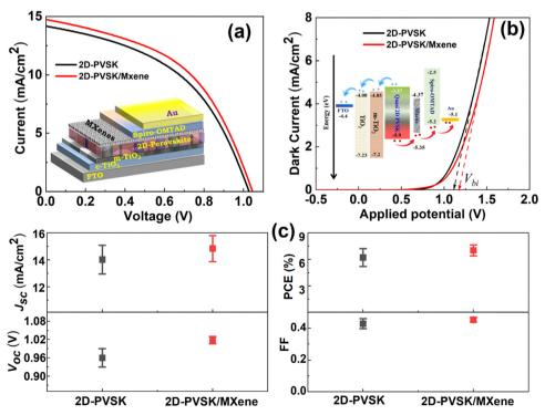
Fig. 3 Current density-voltage curves under (a) light illumination and (b) dark. Inset figures demonstrated a device's structure, and its band energy alignment to show probable charge transfer. (c) Evaluated average parameters for several devices from J-V curves under light illumination.
