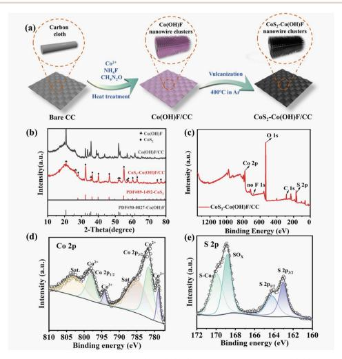
Fig. 1 (a) Schematic illustration showing the preparation of the  $CoS_2$ -Co(OH)F composite on the surface of CC. (b) XRD pattern and XPS spectra of the  $CoS_2$ -Co(OH)F: (c) full, (d) Co 2p and (e) S 2p spectra.
