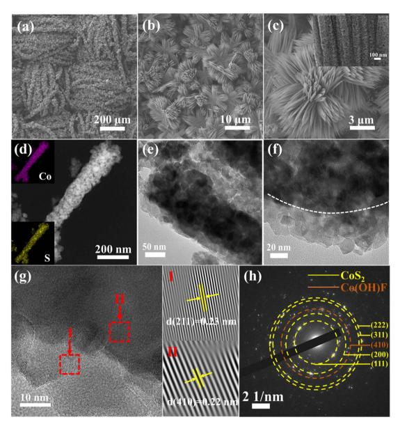
Fig. 2 (a-c) SEM images of CoS<sub>2</sub>-Co(OH)F/CC nanowire clusters at different magnifications. (d) Elemental mapping, (e-q) TEM images, and (h) SAED pattern of the CoS<sub>2</sub>-Co(OH)F nanorod.
