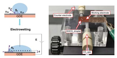
Fig. 5 Illustration of electrowetting (left) and photo of the homemade platform that permits the operando observations of electrowetting during CO<sub>2</sub> electrolysis developed by Gao *et al.* Adapted from ref. 81 with permission from American Chemical Society, copyright 2021.
