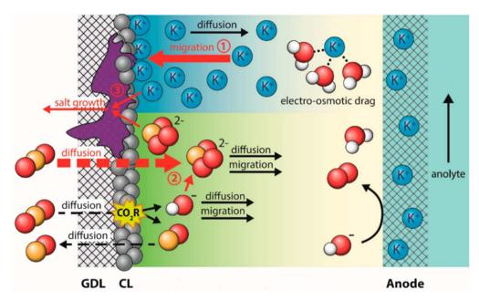
Fig. 6 Schematic of the salt precipitation degrading the GDE together with electrolyte flooding. Reproduced from ref. 96 with permission from American Chemical Society, copyright 2023.
