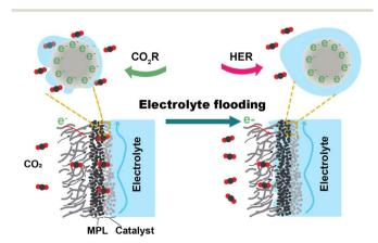
Fig. 1 Illustration of electrolyte flooding in a GDE: the left depicts the ideal conditions of gas and liquid streams within a GDE composed of a microporous layer (MPL) and catalyst during CO<sub>2</sub> electrolysis, while the right side illustrates the microenvironment of a GDE confronting electrolyte flooding
