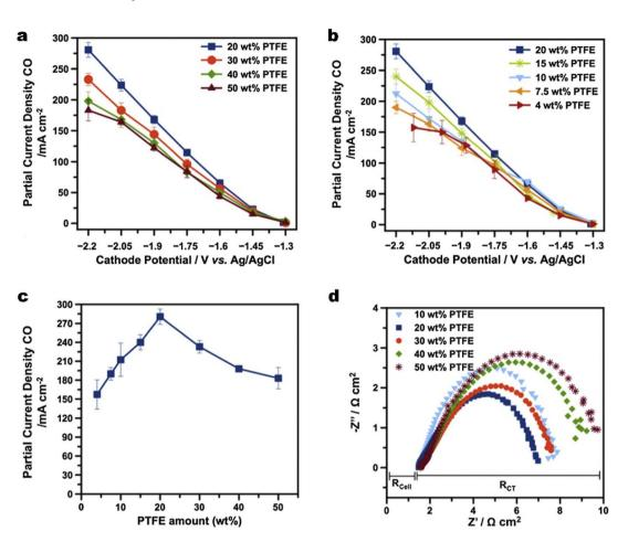
Fig. 11 (a) and (b) Partial current density of CO and  $H_2$  as a function of different potentials for GDEs composed of MPLs with different amounts of PTFE wt%; (c) a comparison of partial current densities of CO for a Ag-based GDE as a function of PTFE content in the MPLs; and (d) the Nyquist plot of electrochemical impedance spectra for the GDEs with different PTFE contents in MPLs. Reproduced from ref. 64 with permission from Elsevier, copyright 2016.
