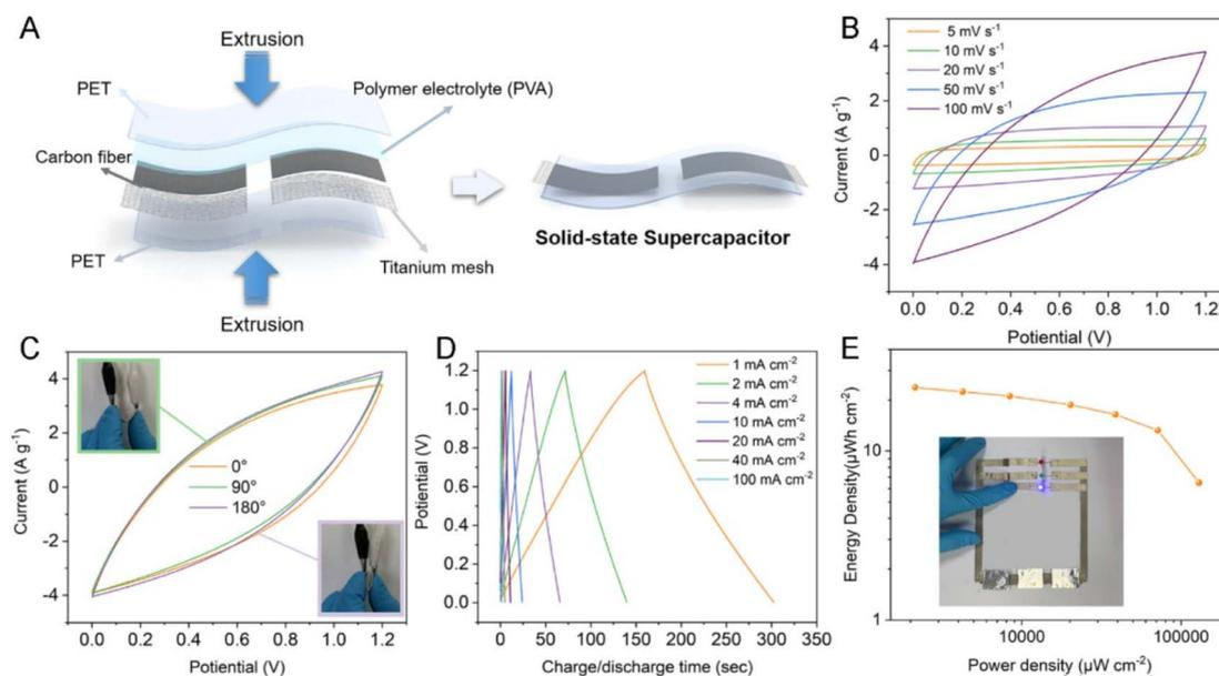
Fig. 16 (A) Preparation of SC; (B) CV curve of device; (C) CV curve of device at different bending angles (inset images show the digital images of bending at  $90^\circ$  and  $180^\circ$ ); (D) GCD curve; and (E) Ragone plot with inset showing a blue LED constructed powered by the device. Reproduced with permission from ref. 57 Copyright (2021), the American Chemical Society.
