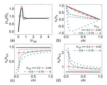
Fig. 8 Shear startup of GCB model WLMs at an applied shear rate of Wi = 5. (a) Shear stress evolution at the inner cylinder (r/H = 0). Normalized velocity (b), number density of species A (c), and number density of species B (d) are shown at five times during the shear stress evolution (O in (a)). Shear stress is normalized by  $G_0$ , velocity by the imposed wall velocity  $v_0$ , and number densities of species A and B by the number density of species A at rest,  $n_{A,0}$ .
