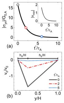
Fig. 7 Relaxation of normalized (a) shear stress and (b) velocity profiles at three times (O in (a)) during flow cessation. Flow achieved steady state before flow was stopped;  $v_0$  is the imposed wall velocity during the preceding shear. Time is normalized by the relaxation time of fluid A,  $\tau_A$ ;  $t^* = t - t_c$  denotes the elapsed time after flow ceases. (a, inset) Shear stress and  $|v_{min}|$  decay with the same time constant.
