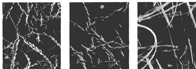
Fig. 23 Original 1965 TEM images of lithium 12-hydroxystearate: (left) D-form, right handed twist, (centre) L-form, left-handed twist, (right) D,L-racemate, no twist. Reproduced from ref. 195 with permission of the American Chemical Society, © 1965.
