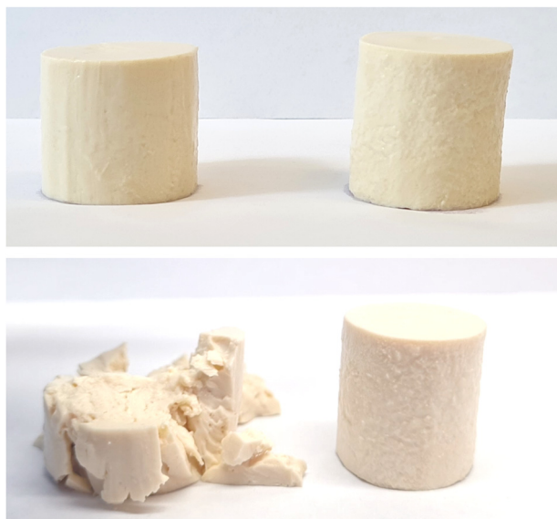
Fig. 3 Fermentation-induced pea protein emulsion gels without TG (left) and with TG (right). The top image shows the gels standing prior to compression, and the lower image shows the gels after compression.
