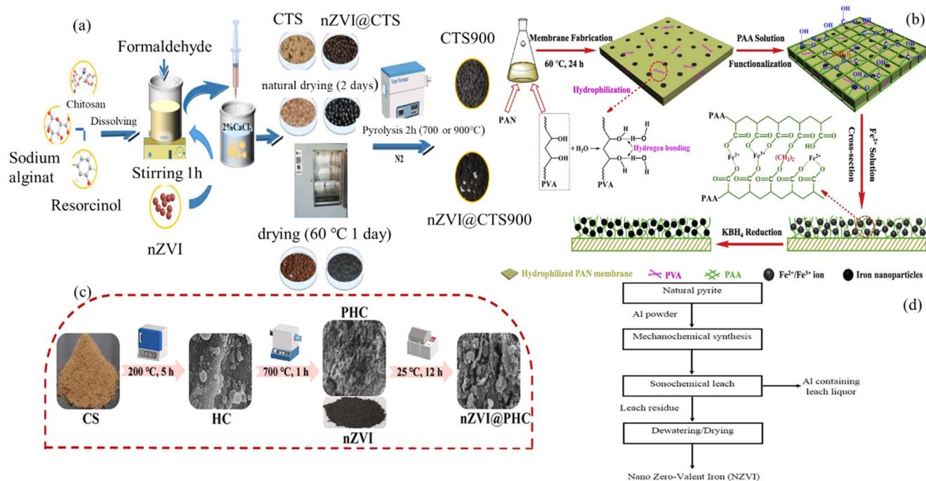
Fig. 1 Process flow of four different nZVI preparation methods (a–d).<sup>22–25</sup>
