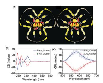
Fig. 7 (A) The overall structures of R/S-Au<sub>3</sub>. Color codes: Au, yellow; P, orange; C, gray. (B) CD spectra of Au<sub>3</sub>[(R)-Tol-BINAP]<sub>3</sub>Cl and Au<sub>3</sub>[(S)-Tol-BINAP]<sub>3</sub>Cl clusters in DCM. (C) CPL spectra of R-Au<sub>3</sub> and S-Au<sub>3</sub> assemblies in 70% n-hexane. (Reproduced from ref. 45 with permission from John Wiley and Sons, Copyright 2017).
