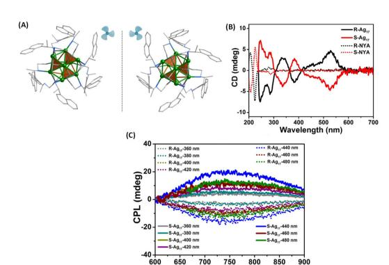
Fig. 6 (A) The aromatic moieties of the ligands resemble a triblade fan when viewed parallel to the  $C_3$  axis. Color code: Ag, green; N, blue; C, gray. All hydrogen atoms have been omitted for clarity. (B) CD spectra of R/S-Ag<sub>17</sub> (solid trace) and ligands R/S-NYA (dotted trace) in solution and (C) CPL spectra of R/S-Ag<sub>17</sub> at different excitation wavelengths in the solid state. (Reproduced from ref. 46 with permission from the American Chemical Society, Copyright 2021).
