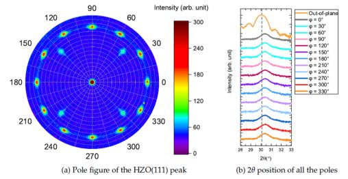
Fig. 4 Panel (a) shows the pole figure of the HZO (111) peak of a 10 nm HZO film on a single crystal STO substrate. The radial angle  $\chi$  ranges from 0° up to 85° and the azimuthal angle  $\phi$  ranges from 0° to 359°. Panel (b) shows the 2 $\theta$  position of each pole. The dashed line is drawn at the position of the out-of-plane (111) pole as a guide to the eye.
