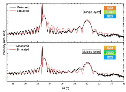
Fig. 3 Both graphs show the experimental data in black and the simulated data in red. The top graph shows the simulation for single layers. The bottom graphs show the results of the simulation in case the LSMO and the HZO layers are split up into three and two sublayers, respectively.
