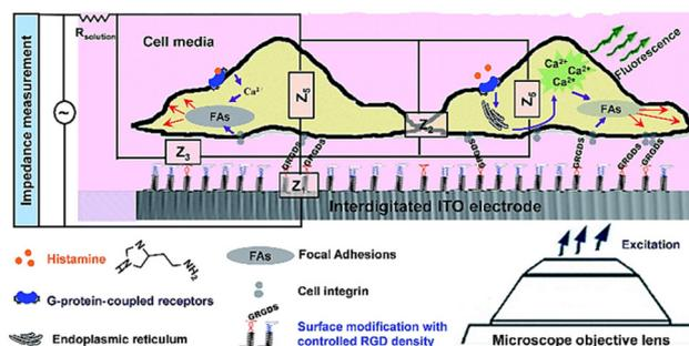
**Fig. 19** The simultaneous dual sensing platform was developed to gather more detailed data on how cells react to soluble stimuli when self-assembling adhesive ligands are present on interdigitated indium tin oxide (ITO) surfaces. The displayed content reproduced from ref. 75. Copyright 2017 Royal Society of Chemistry.
