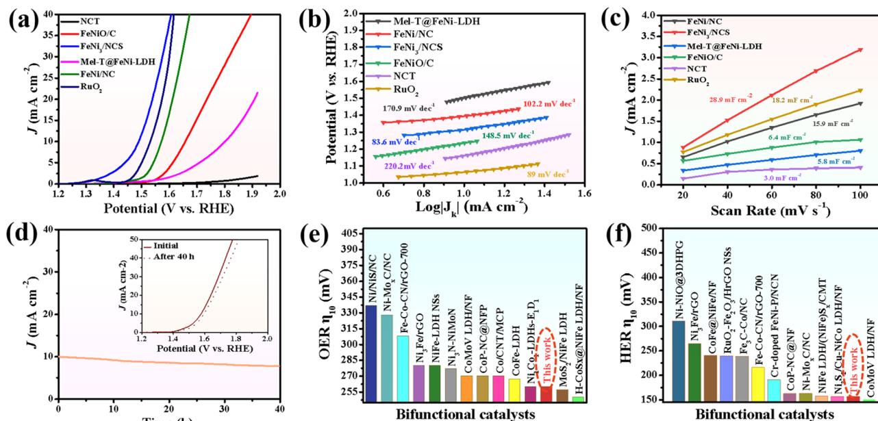
Fig. 3 (a) OER LSV profiles, (b) Tafel slopes, and (c)  $C_{dl}$  of FeNi<sub>3</sub>/NCS, NCT, FeNiO/C, FeNi/NC, Mel-T@FeNi-LDH and RuO<sub>2</sub>. (d) Amperometric  $i-t$  of FeNi<sub>3</sub>/NCS at 10 mA cm<sup>-2</sup> (inset: the polarization curve of FeNi<sub>3</sub>/NCS after  $i-t$  measurement); comparison of (e) OER and (f) HER overpotential of this work and reported FeNi-containing electrocatalysts.
