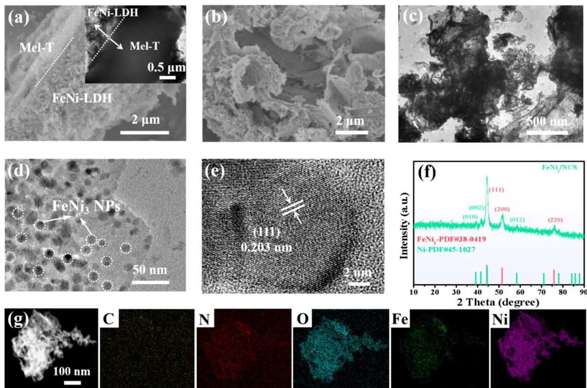
Fig. 1 SEM and inset TEM images of (a) Mel-T@FeNi-LDH; (b) SEM, (c and d) TEM, (e) HRTEM images, (f) XRD pattern and (g) elemental mapping images of FeNi<sub>3</sub>/NCS.
