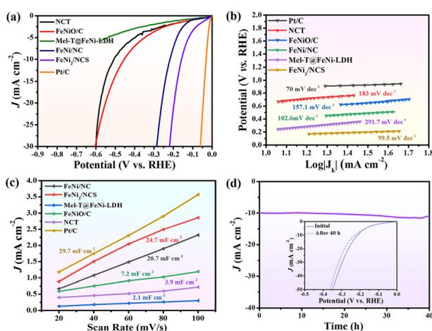
Fig. 4 (a) HER LSV profiles, (b) Tafel slopes, (c)  $C_{dl}$  of NCT, FeNiO/C, FeNi/NC, Mel-T@FeNi-LDH, FeNi<sub>3</sub>/NCS, and Pt/C. (d) Amperometric  $i-t$  curve of FeNi<sub>3</sub>/NCS at  $10\text{ mA cm}^{-2}$  (inset: the polarization curve of FeNi<sub>3</sub>/NCS after  $i-t$  measurement).
