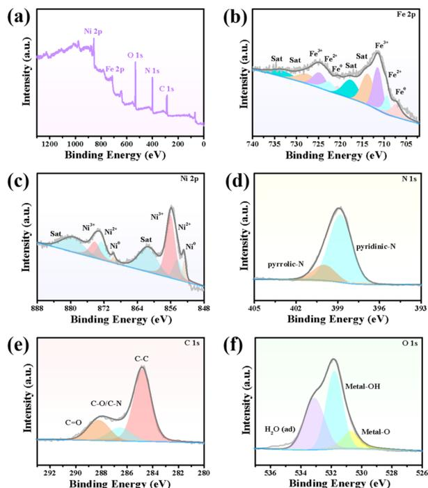
Fig. 2 (a) Full survey XPS spectrum and high-resolution XPS spectra of (b) Fe 2p (c) Ni 2p, (d) N 1s, (e) C 1s, and (f) O 1s of FeNi<sub>3</sub>/NCS.
