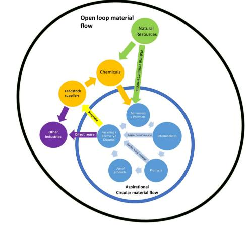
Fig. 1 Simplified example of material flow in the Composites Industry.
