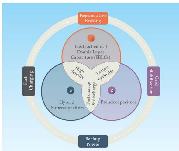
Fig. 6 Supercapacitors' types, functions and advantages representation.
