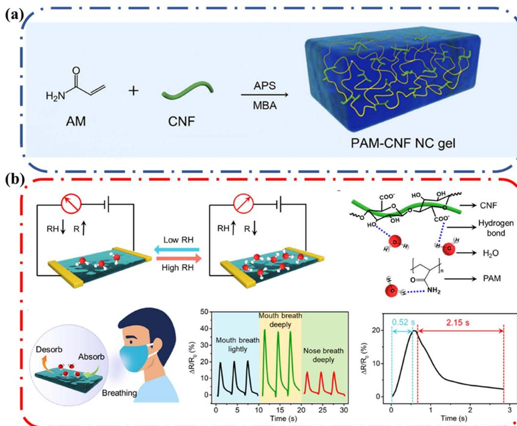
Fig. 17 (a) Schematic illustration of the fabrication of the PAM-CNF NC gel *via in situ* radical polymerization (b) schematic illustrating the humidity sensing mechanism of the CS-NC gel, the formation of hydrogen bonds between water and CNF, as well as water and PAM, schematic diagram of breath monitoring and resulting relative resistance changes of CS-NC sensors under different breath conditions. Reprinted with permission from Yu *et al.*<sup>77</sup> Copyright 2022 American Chemical Society.
