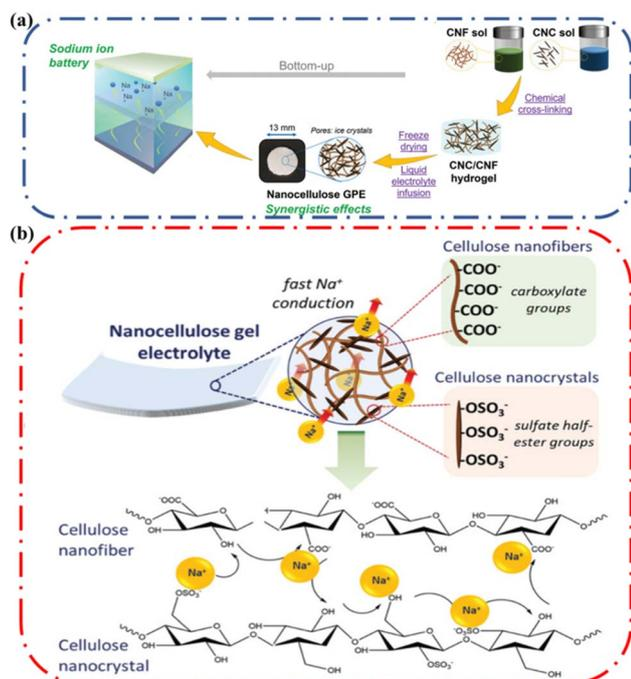
Fig. 10 (a) Schematic representation of the nanocellulose gel electrolyte fabrication. (b) Schematic illustration of the proposed  $\text{Na}^+$  conduction mechanism across the nanocellulose Gel Polymer Electrolyte (GPE). Reprinted with permission from Mittal *et al.*<sup>62</sup> Copyright 2022 Wiley.
