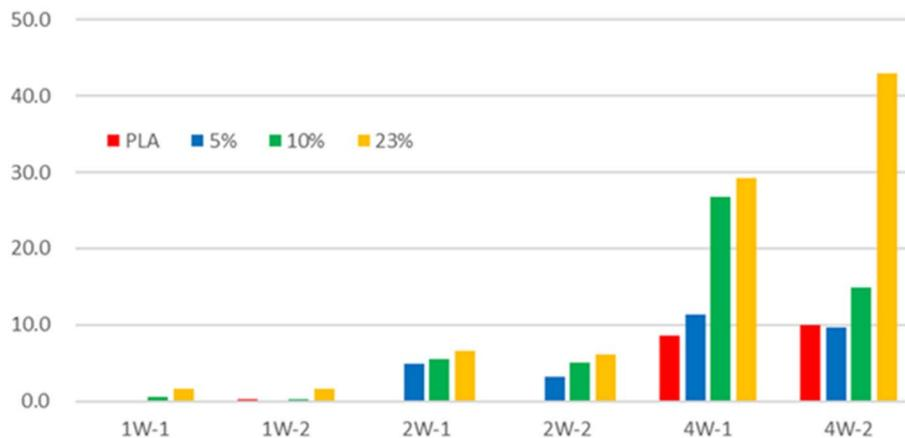
Fig. 4 Biodegradability test result. It can be seen that biodegradability increased as the content of nanocellulose increases in the PLA-nano-cellulose composite material.<sup>49</sup>
