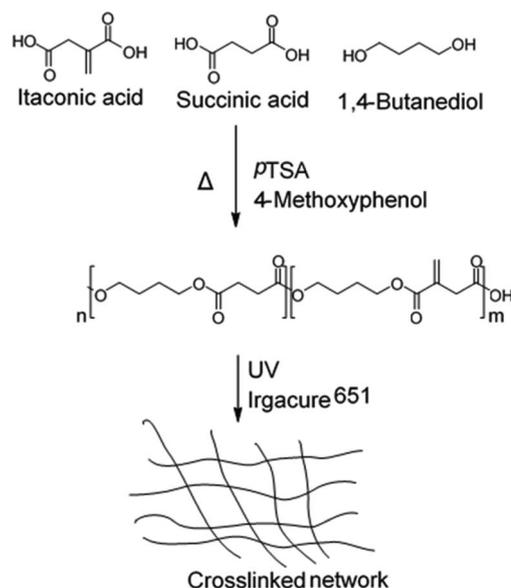
Fig. 26 Synthesis and crosslinking of renewable polyesters containing itaconic acid, succinic acid, and 1,4-butanediol.<sup>114</sup>
