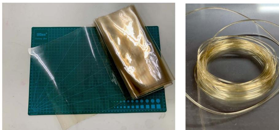
Fig. 9 Biomass biodegradable film (Left) and yarn and fiber (Right) made of cellulose-based biodegradable plastic.<sup>58</sup>
