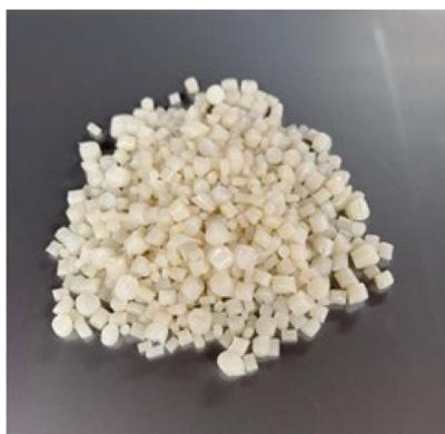
Fig. 7 Starch-based biodegradable plastic prepared with twin-axis extruder composed of 100% biomass.<sup>54</sup>
