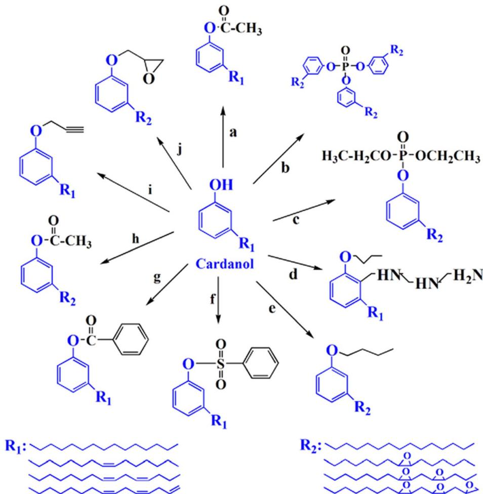
Fig. 29 Chemical structure of cardanol-based plasticizer.<sup>119–121</sup>
