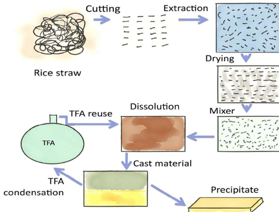
Fig. 41 Synthesis of bioplastics from rice straw (TFA: trifluoroacetic acid).<sup>180</sup>
