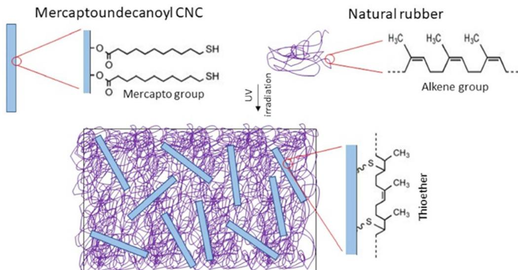
Fig. 32 Illustration of the thiolene coupling reaction between natural rubber and modified cellulose nanocellulose in nanocomposite.<sup>156</sup>
