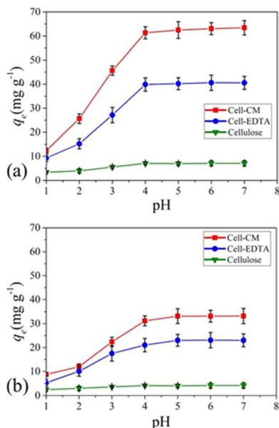
Fig. 15 Adsorption efficiencies of extracted cellulose, cell-EDTA (ethylene diamine tetra acetic acid-modified nanocellulose), and cell-CM (carboxy methyl group-modified nanocellulose) for (a)  $\text{Pb}^{2+}$  and (b)  $\text{Cd}^{2+}$  in the pH range of 1–7. Conditions for adsorption: concentration of  $\text{Pb}^{2+}$  or  $\text{Cd}^{2+}$  =  $100 \text{ mg L}^{-1}$ , at room temperature for 90 min.<sup>81</sup>
