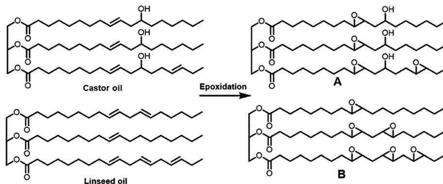
Fig. 20 . Vegetable oil-based epoxy monomer derived from castor oil and linseed oil.<sup>93,94</sup>
