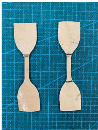
Fig. 33 Dumbbell test piece of (Left) natural rubber and (Right) natural rubber nano cellulose composite material.<sup>180</sup>
