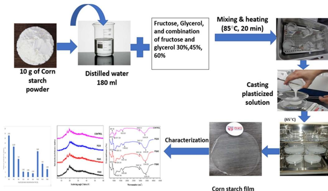
Fig. 6 Procedure for the preparation of starch-based bioplastic by the casting method.<sup>51</sup> Starch bioplastic was prepared by mixing corn starch, water and plasticizer.
