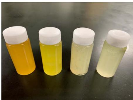
Fig. 16 Nano cellulose dispersion in vegetable oil. From (Left), sesame oil, olive oil, castor oil, soy bean oil.<sup>83</sup>
