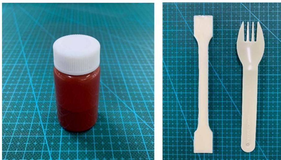
Fig. 35 Biomass biodegradable paint (Left) and plastic (Right) with anti-bacterial activity.<sup>160</sup>
