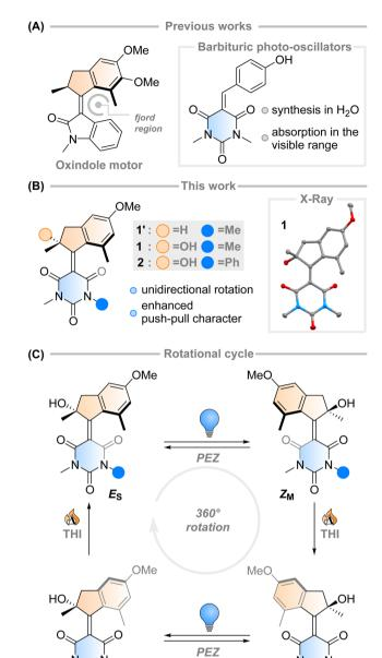
Fig. 1 (A) Previous literature examples that led to the Feringa-type light-driven molecular motor presented in this work. The molecule is based on a charge-transfer oxindole structure and barbituric acid-based photo-oscillators. (B) This work, an investigation of barbituric acid-based molecular motors 1 and 2 (X-ray structure of 1: non-H atoms represented as 50% probability ellipsoids, H-bond evidenced for clarity). (C) Proposed rotational cycle of motors 1 and 2.
