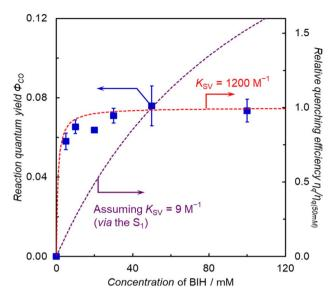
Fig. 11 Plot of the  $\Phi_{CO}$  versus the initial concentration of BIH in the photocatalytic CO<sub>2</sub> reduction (Xe lamp, 420 nm, 3.6  $\times$  10<sup>-8</sup> einstein per s) using DMA-TEOA (4:1 v/v) solutions containing ZnP-5Bpy= Re<sup>Br</sup> (0.05 mM). The quenching efficiency relative to  $\eta_q$  at [BIH] = 50 mM was calculated using  $\eta_q = [\text{BIH}]K_{SV}/(1 + [\text{BIH}]K_{SV})$ .
