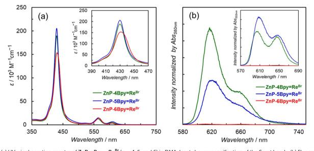
Fig. 4 (a) UV-vis absorption spectra of ZnP-nBpy=Re<sup>Br</sup> (n = 4, 5, and 6) in DMA. Inset shows magnification of the Soret bands. (b) Fluorescence spectra of ZnP-nBpy=Re<sup>Br</sup> (n = 4, 5, and 6) in Ar-saturated DMA ( $\lambda_{ex}$  = 560 nm) at 298 K. Inset shows spectra in Ar-saturated toluene ( $\lambda_{ex}$  = 553 nm) at 298 K. The fluorescence spectra were normalized with absorbance at the excitation wavelength.
