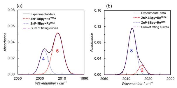
Fig. 15 IR spectra (solid line) of the equilibrated mixture of (a) ZnP-5Bpy=Re<sup>DMA</sup> and ZnP-5Bpy=Re<sup>TEOA</sup>, and (b) ZnP-6Bpy=Re<sup>DMA</sup> and ZnP-5Bpy=Re<sup>DMA</sup> and 6Bpy=Re<sup>TEOA</sup> in DMA-TEOA (400:1 v/v) with the fitting curves (dotted lines). Concentrations of the dyads: 9 mM.
