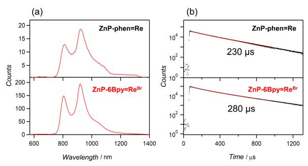
Fig. 5 (a) Phosphorescence spectra of ZnP-phen—Re and ZnP-6Bpy—Re<sup>Br</sup> in Ar-saturated DMA ( $\lambda_{ex} = 405$  nm) at room temperature. The spectra were recorded with delay time > 90 μs after the excitation pulse. (b) Phosphorescence decay profiles (semilog plot) of ZnP-phen—Re and ZnP-6Bpy=Re<sup>Br</sup> in Ar-saturated DMA ( $\lambda_{ex} = 405$  nm) at room temperature, monitored at 800 and 920 nm. The decay profiles were fitted with one component (red lines)
