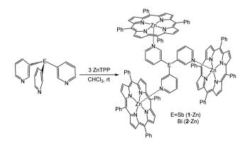
**Scheme 1** Synthesis of the capsules  $\{[Sb(3-py)_3]\cdot (ZnTPP)_3\}$  (1·Zn) and  $\{[Bi(3-py)_3]\cdot (ZnTPP)_3\}$  (2·Zn).
