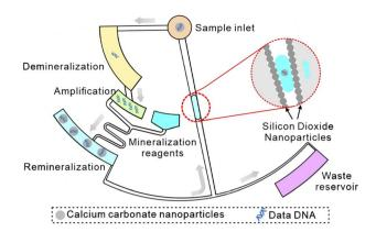
Scheme 1 Schematic of a CD microfluidic platform for non-destructive information extraction from mineralized DNA data.
