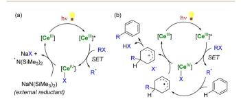
Scheme 6 Schematic (photo)catalytic cycle involving the Ce(IIII/IV) couple with (a) or without (b) the use of an external sacrificial reductant. 91,94
