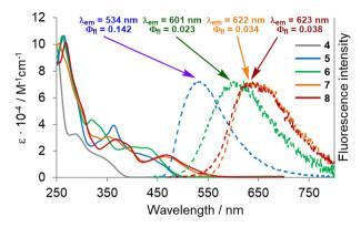
Fig. 6 UV-vis absorption spectra (solid lines) and fluorescence spectra (dashed lines) of dyes 4–8 measured in dichloromethane.
