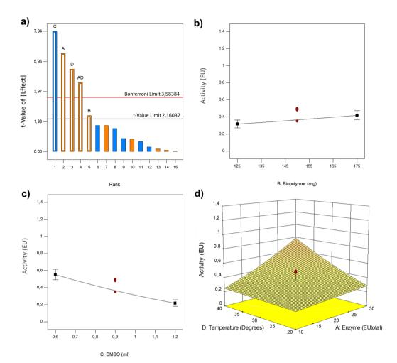
Fig. 2 Factorial design analysis. (a) Pareto chart ((A) enzyme; (B) biopolymers; (C) DMSO; (D) temperature; in orange factors with positive effects; in blue negative effects); (b) effect of the factor biopolymers (mg); (c) effect of the factor DMSO (mL); (d) effect of the interaction between temperature and enzyme charge.
